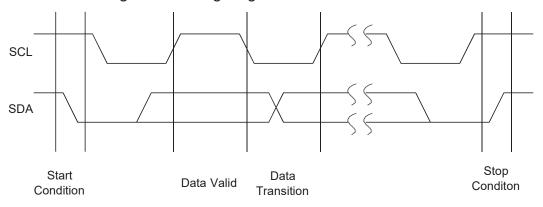
Figure 1: Timing diagram for START and STOP condition
